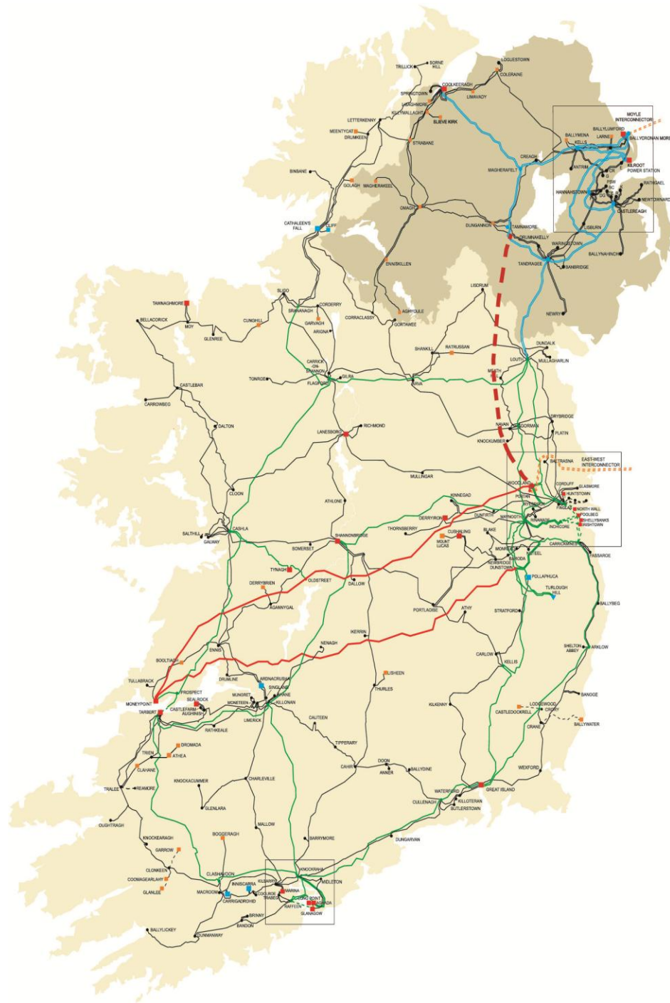
Figure 4.12: Map Showing Transmission Network and Proposed Interconnector
